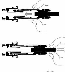
The latching of plug into the receptacle is achieved by a simple axial pushing on the outer shell.
