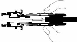
To unmate the plug from the receptacle, just pull the outer shell axially.
