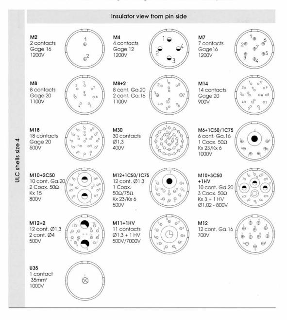
Insulation resistance size I, III, IV and V :  $\geq$  5000 Megohms under 500 Vdc (Unmated connectors)
