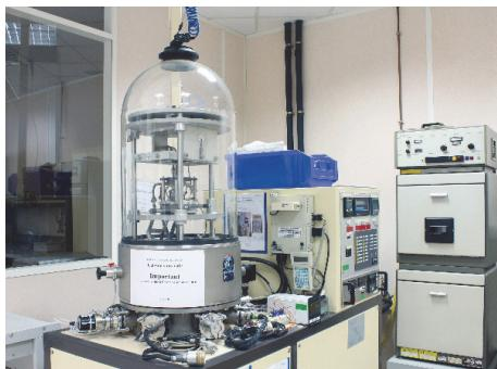
Vacuum bell for robotic operating testing
