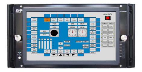
The ACU-22JDA is fitted with an integrated 15 inch touch screen display flanked by hand positioning controls for the antenna mode and position. The default legacy display is an antenna control display that is familiar to many telemetry engineers in terms of look and functionality, this may be switched at any time to the full VuSoft environment as required.
