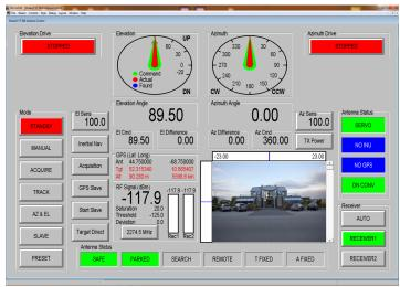
The ACU-22JDA may be remotely monitored and controlled as required via both external Ethernet and external RS232 links.
